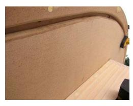
You will be drilling 8 holes evenly spaced around the rail, these holes should be 1 1/8" in from the inside edge of the rail. Using a  $\frac{3}{4}$ " spade drill bit, drill 8 holes to a depth of  $\frac{1}{2}$ " -  $\frac{3}{4}$ ". Using a  $\frac{5}{16}$ " wood drill bit, drill through the remaining depth of the rail and through the table.
