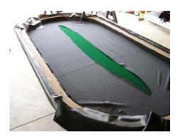
Gently pull the vinyl at the middle of one of the sides, so the cut that you put down the middle starts to pull open about 3". Then put a staple into the inside edge. Repeat on other side. The middle cut should be about 6" wide in the center.
