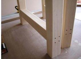
Wipe off any excess glue. Fill the screw holes with wood filler. Once the glue and wood filler is dry, sand those areas smooth with the orbital sander.
