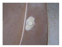
Remove the rail from the table. Gently pound each of the T-bolt nuts into the holes. Put a  $\frac{3}{4}$  " piece of board under the lip of the rail to provide support, so the rail is not damaged. Secure rail back on the table, by screwing in place with all 8 bolts. Fill in the  $\frac{3}{4}$  " holes with wood filler. Sand when dry.
