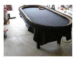
Start at the middle of a round end. Pull the vinyl up and over to the inside edge and put 1 staple in place. Go to the other end and do the same thing. Take the utility knife and cut down the center of the vinyl inside of the rail. Make the cut about 5' in length parallel to the straight sides of the rail. (The reason for this is that you will be pulling the vinyl out on the sides which will then help it go around the round ends.)
